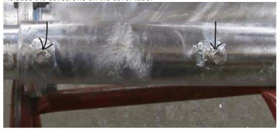
Release the cover tube from the pump housing and from the gearbox housing. Rinse cleanly inside the cover tube.
