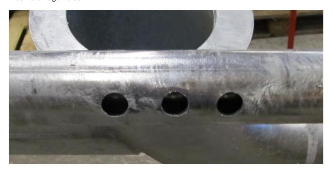
If this does not help, the cover tube is most likely full of dried slurry. Release the set screws on the cover tube.
